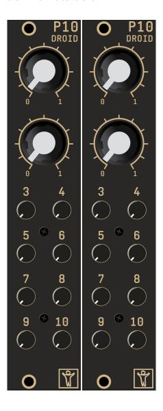
The P10 controller has two big pots (the same as the P2B8 controller) and eight small pots. That makes a total of 10 pots, which are all behaving in the same way. They are numbered from 1 to 10, so if your P10 would be the first in the chain, these pots are adressed in a DROID patch by
