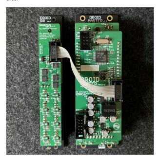
The G8 version 2 has two connectors. Here use the right one labelled "Master":
