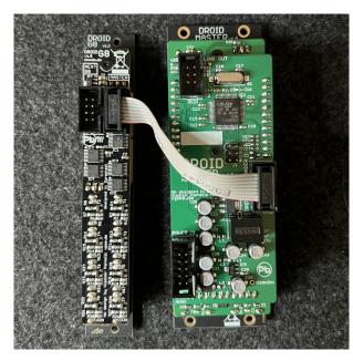
To create a chain, wire the master to the "Master" input of the first G8, which must be version 2. Then wire the other connector of this G8 to the "Master" input of the second G8 and so on. No termination jumper is needed. The last G8 in the chain can either be version 1 or version 2.
