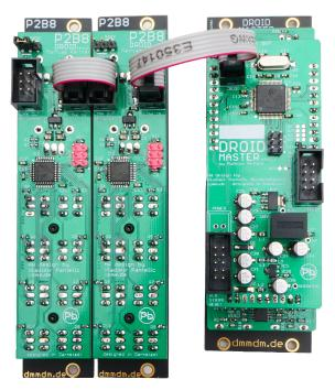
If you switch on your system after connecting the controllers, those with LEDs should make a short power up animation. This does *not* mean that they are wired and jumpered correctly, though. To make a real test, you need to prepare a DROID patch, as you will see below.
