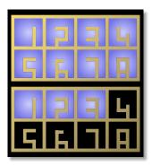
When the end is reached - this time at O8 - and you *now* release the button, the DROID enters the maintenance mode. If you let go the button before this you go back into normal operation.
