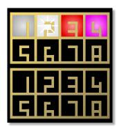
A *long* press of the button selects the item the cursor is currently at. It starts an animation on the LEDs of O1 ... O8 in the same color as the selected item (in this case calibration mode):
