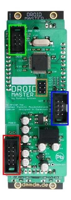
Do not mix up the connectors! This will destroy your electronics. Do not force in cables in the wrong orientiation or with the wrong number of pins! Do not attach anything to the programming port.
