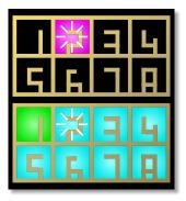
Now proceed to the second pair of jacks and connect input 2 to output 2. Do this until all eight channels are green. DROID will then automatically end calibration and start normal operation.
