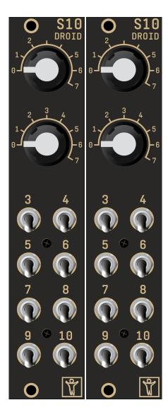
The S10 controller has ten switches. They have the register abbreviation **S**. The first two are rotary switches and have eight positions. They output the discrete numbers **0**, **1**, ... **7**. The small switches just have three positions: **0** (down), **1** (center) and **2** (up).
