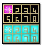
Now use a patch cable and connect input 1 to output 1. DROID now tries out different output voltages and measures them by means of the precision ADC of input 1. This information is being used for the exact calibration. The result of the calibration is saved to the DROID's internal flash memory.
