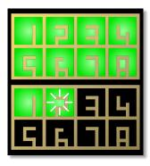
In case of an error, all 16 LEDs blink in one color. If all LEDs blink **yellow**, the firmware file is missing (which is strange, because it was there at the beginning):
