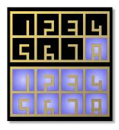
When the blue LEDs reach I1, continue holding the button. DROID restarts. Still hold the button. Now the animation of the blue LEDs starts in the opposite direction:
